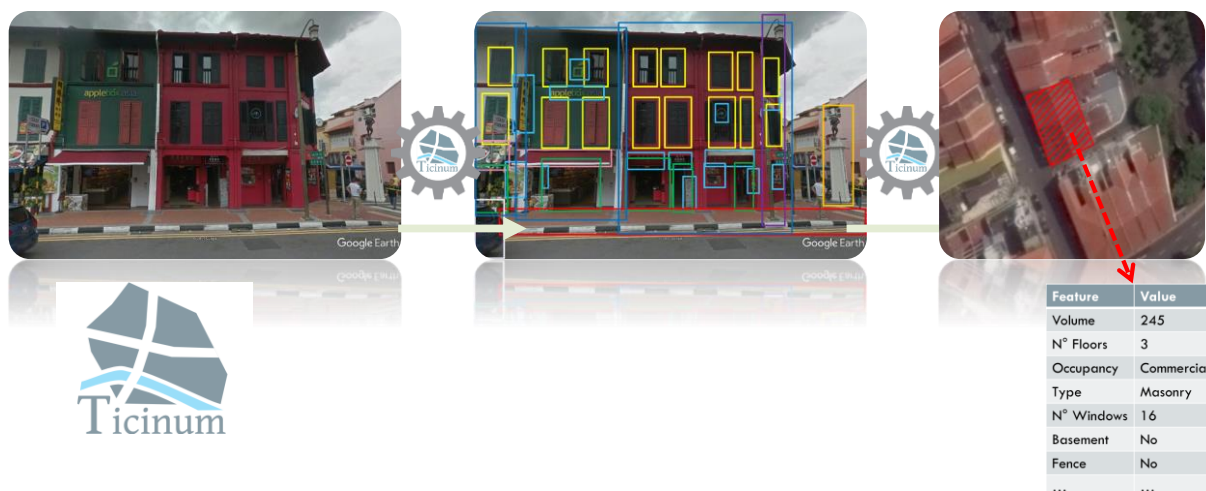
Figure 2.1 The CountFloor service of Ticinum can automatically extract building features by analysing street-level pictures
