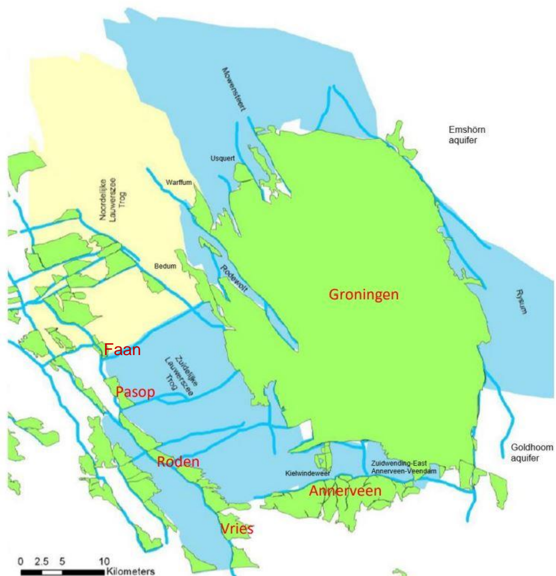
Figure 6: The Groningen field and connected aquifers (in blue) and gas fields (in green).
