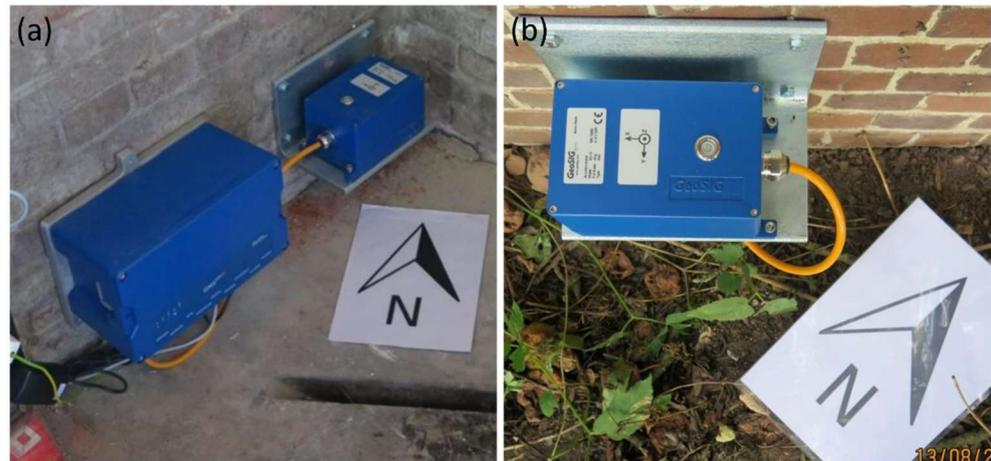
Figure 3 (a) Geosig sensor near a stiff corner on the outside of a building, and (b) a Geosig sensor near the stiff corner inside, the large box to the left is the recorder, the small box to the right is the sensor.
