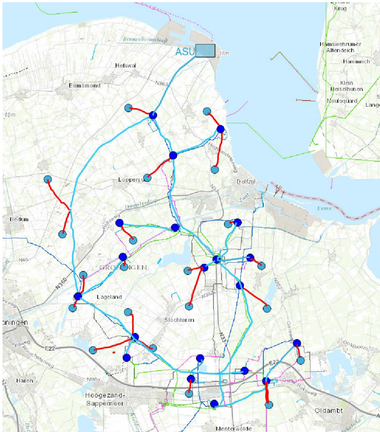
Figure 12.20 Plot lay-out of the ASU plant, N 2 injection facilities, NRU's wells and pipelines in the Groningen province
